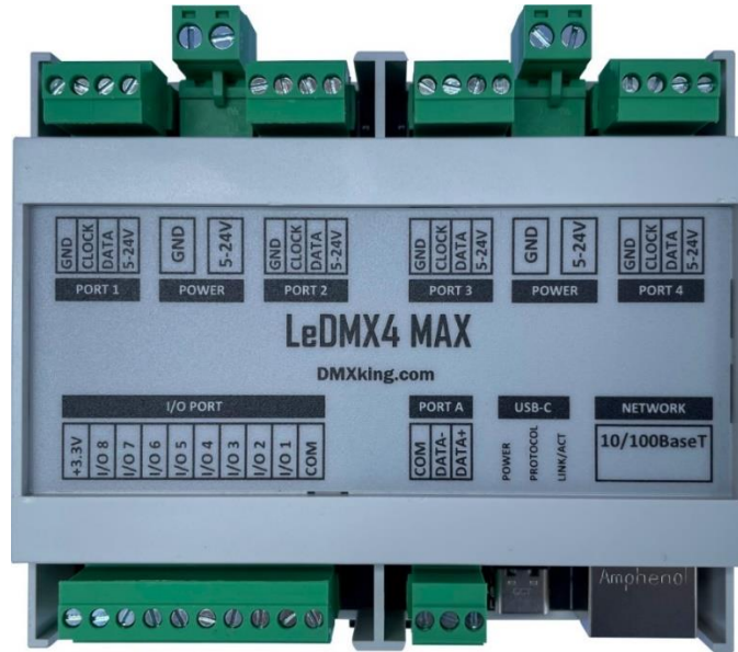
LeDMX4 MAX I/O Port 8x trigger inputs **Reversed I/O designations shown in this image
