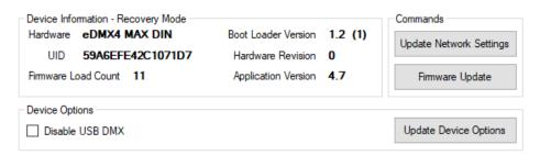
For applications where it is undesirable to have USB device configuration or USB DMX functionality available the USB port can be disabled with Device Option **Disable USB DMX**.
