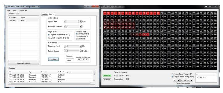
The DMX Display utility works with any manufacturers Art-Net hardware and can be useful for diagnostics and simple testing of DMX512 fixtures.
