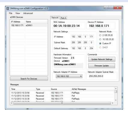
Before starting the eDMX Configuration utility please ensure your computer has appropriate IPv4 network settings, for example IP 192.168.0.100 Subnet 255.255.255.0 Gateway 192.168.0.254.
